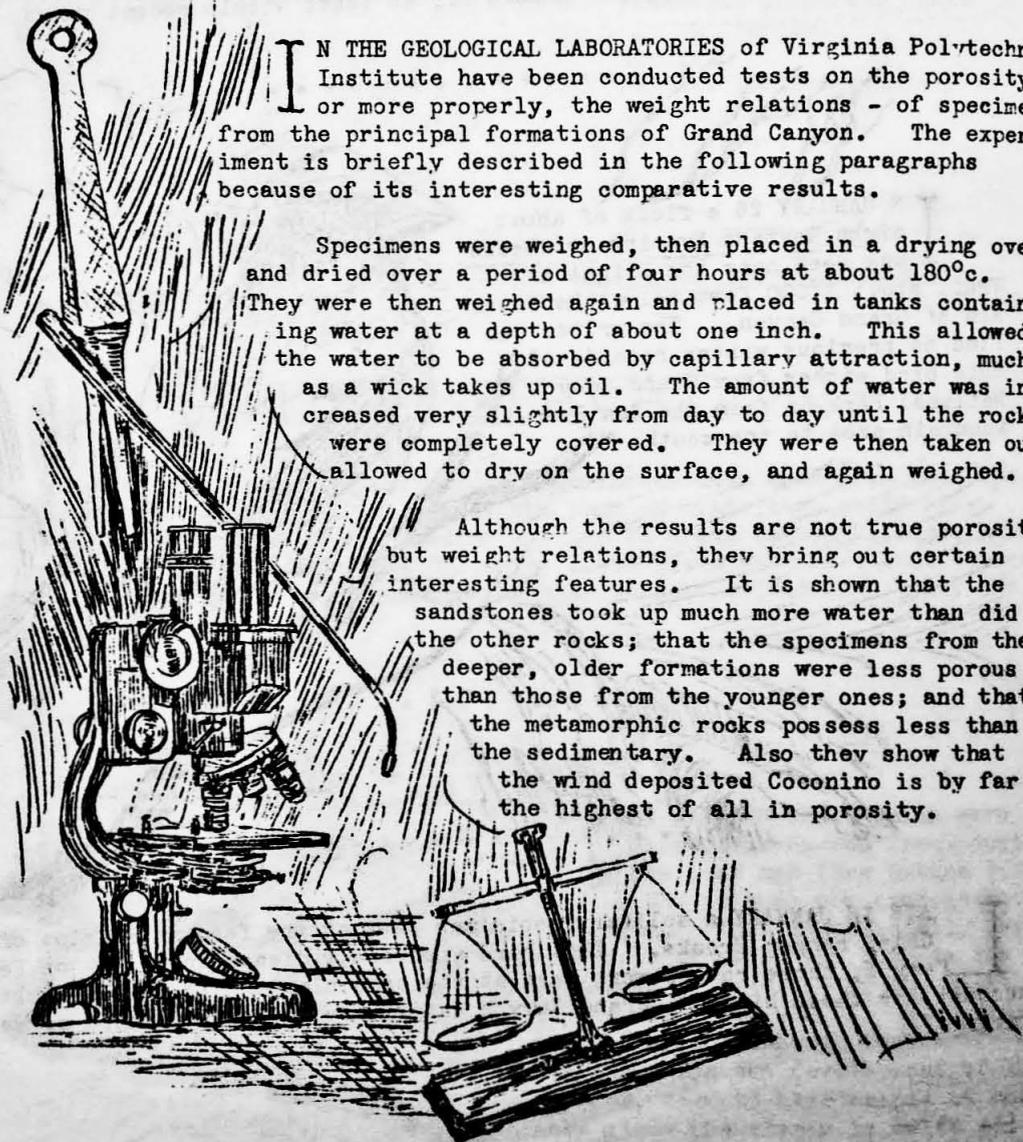
IN THE GEOLOGICAL LABORATORIES of Virginia Polytechnic Institute have been conducted tests on the porosity - or more properly, the weight relations - of specimens from the principal formations of Grand Canyon. The experiment is briefly described in the following paragraphs because of its interesting comparative results.
